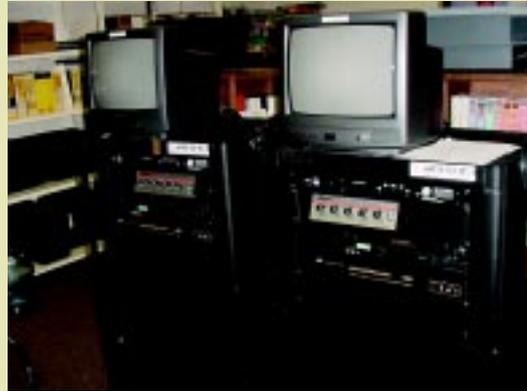
from 18 remote “mini” head ends. Specifically, each video programming cart is equipped with a Canon camcorder, Bogen fluid head tripod, Sony VCR, Electro-Voice handheld microphone, Shure four-channel mic mixer and Blonder Tongue sub-band fixed agile AV modulator.
